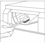
Pull the drawer to remove (slightly at first till the stop, then pull hard).
